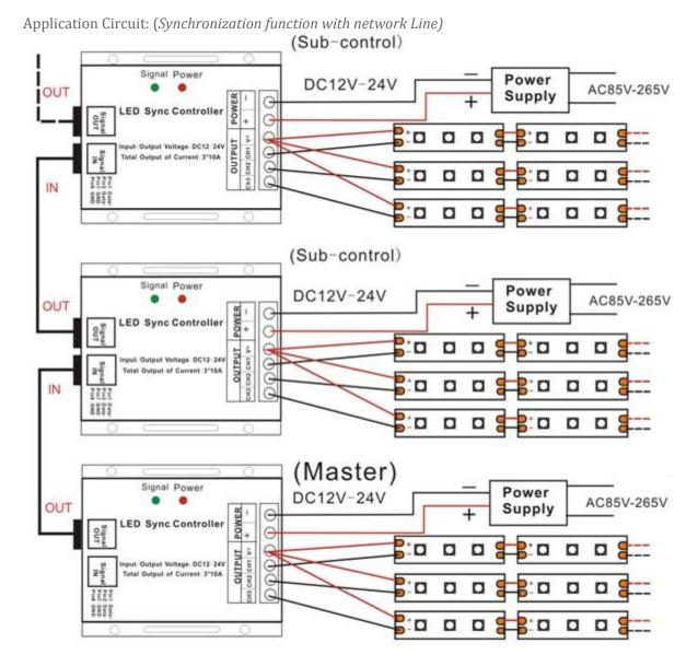
Tips: The green signal indicator light will flash with proper communication.
